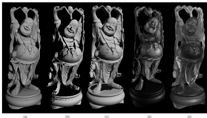
FIGURE 14.12: 3D Fax of a statuette of a Buddha. From left to right: photograph of the statuette; range image; integrated 3D model; model after hole filling; and physical model obtained via stereolithography. Courtesy of Marc Levoy. Reprinted from "A Volumetric Method for Building Complex Models from Range Images," by B. Curless and M. Levoy, Proc. SIGGRAPH, (1996). © 1996 ACM, Inc. http://doi.acm.org/10.1145/237170.237269 Reprinted by permission..
