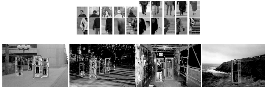
Fig. 3.2 Mohan et al. use SVM's to find major body parts (left arm, right arm, head/shoulders and legs) as in the training examples shown on the top . They then use these SVM's to search frames for components; the response of all part SVM's in each window is pooled and then presented to an SVM which identifies whole figures. On the bottom , examples showing good detects; the whole body window is outlined with lines, and the part windows with dashed lines. Figure from "Example-Based Object Detection in Images by Components", Mohan et al. , IEEE T-PAMI, 2001, © 2001 IEEE.
