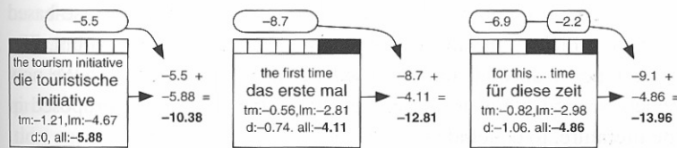
Figure 6.11 Combining probability score and future cost: While the probability score alone may be misleading, adding an estimate of the expected future cost gives a more realistic basis for pruning out bad hypotheses. Here, the hypothesis that tackles the hard part of the sentence the tourism initiative has the worse score (-5.88 against -4.11, -4.86), which is offset by a cheaper future cost estimate (-5.5 against -8.7, -9.1), resulting in an overall better score than the two competing hypotheses that cover simpler parts of the sentence (-10.38 against -12.81, -13.96).
