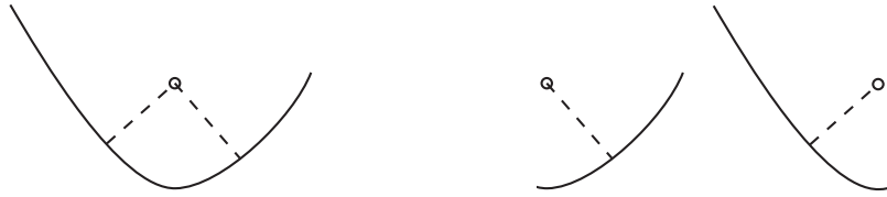
FIGURE 14.3: There can be more than one point on a curve that looks as if it is closest to a token. This makes fitting curves to points very difficult. On the left , a curve and a token; dashed lines connect the token to the two points on the curve that could be closest. The dashed line from token to curve and the tangent to the curve are at right angles for each of the two points on the curve. Center and right show copies of part of the curve; for each, the closest point on the segment to the token is different, because part of the curve is missing. As a result, no local test can guarantee a point is closest – all candidates must be checked.
