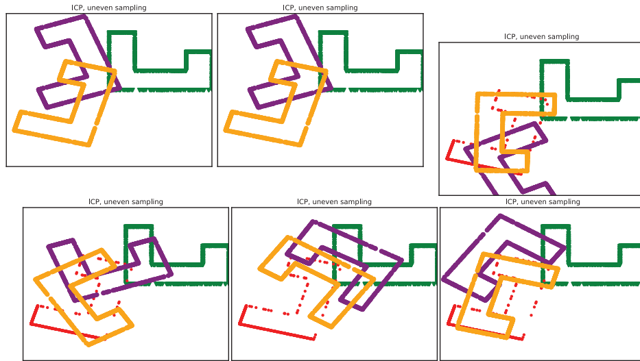
FIGURE 16.7: If the two shapes that have been sampled differently, ICP can produce poor results. The green (upward pointing, to the right) u shape must be transformed to lie on the red (sideways pointing, to the left) u shape. The initial transformation is shown by the purple shape. The ICP result is shown in orange . The two offset cases are successful; the others are not.
