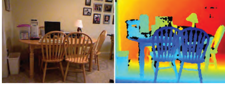
FIGURE 19.6: An example of an RGB image registered to a depth map. The depth map was obtained with a Kinect device. Bluer points are closer, redder are further away. Notice a scattering of black points, which correspond to locations where the Kinect could not determine depth. These tend to occur at the outlines of objects, but can be elsewhere. They are often a result of shadowing effects or specular reflection at the surface. These effects mean some care is required to get normal estimates, as derivatives may be unreliable. Image credit: The images come from the very well known NYUV2 dataset, published at https://cs.nyu.edu/~fergus/datasets/nyu_depth_v2.html .
