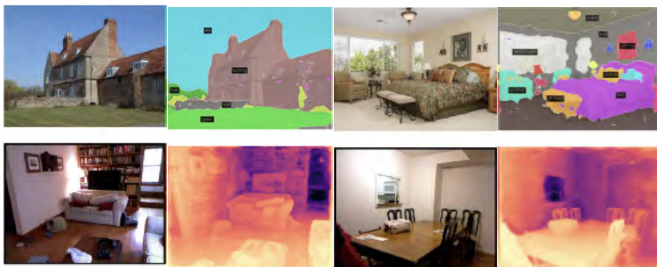
FIGURE 23.7: DINOv2 features are learned without labels, dense, and able to predict depth and segmentation from single images. Top row shows pairs of (image, semantic segmentation). Bottom row shows pairs of (image, depth). In each case, the prediction is obtained with a simple linear decoder applied to frozen DINOv2 features. Image credit: Part of Figure 3 of “ DINOv2: Learning Robust Visual Features without Supervision ”, Oquab et al, 2024
