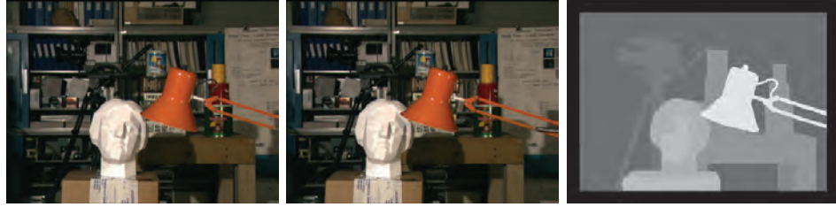
FIGURE 33.5: Two frames (3 and 5) from a well known sequence of five frames, the Tsukuba dataset. On the right , the known ground truth disparity in the coordinate system of frame 3. Image credit: Images from the Middlebury dataset at https://vision.middlebury.edu/stereo/data/ , originally described in Y. Nakamura, T. Matsuura, K. Satoh, and Y. Ohta. Occlusion detectable stereo—occlusion patterns in camera matrix. In CVPR , pages 371–378, 1996.
