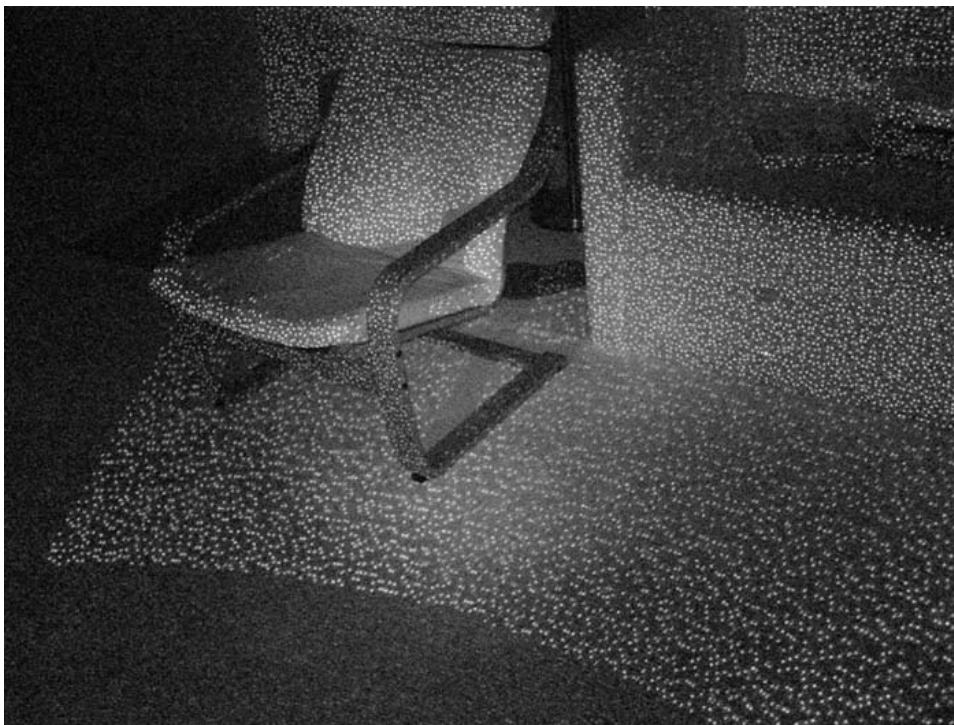
FIGURE 33.10: A pattern of random dots projected by the projector in a Kinect device. The projector slide is known, and the camera can estimate depth by matching as in a random dot stereogram. The dots are in infrared, so not visible to the user. Image credit: An image published at https://bbzipo.wordpress.com/2010/11/28/kinect-in-infrared/ by
