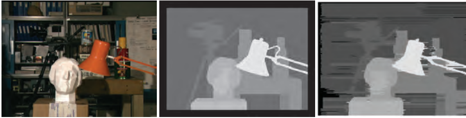
FIGURE 33.6: Dynamic programming based matches produce characteristic streaking errors in the estimated disparity. Left, frame 3 of the Tsukuba sequence (Figure 33.5); center, the ground truth disparity; and right, an estimate from a dynamic programming based method. Image credit: disparity estimate is part of Figure 17 of A Taxonomy and Evaluation of Dense Two-Frame Stereo Correspondence Algorithms, D. Scharstein and R. Szeliski, 2001
