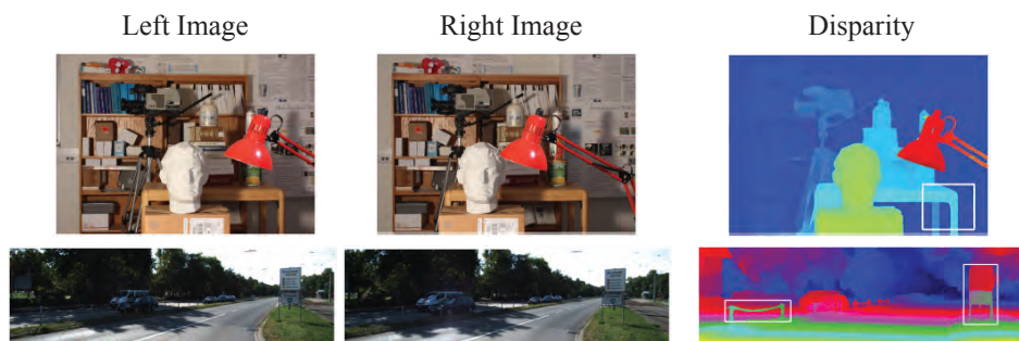
FIGURE 36.5: Refining a disparity estimate using residuals produces strong qualitative results. The figure shows left and right images and disparity maps obtained like this. Note the absence of the spatial noise in disparity (compare the top row with Figures 33.5; 33.6; and 33.7). Image credit: Parts of Figure 6 and 7 of Z. Liang et al., "Stereo Matching Using Multi-Level Cost Volume and Multi-Scale Feature Constancy," in IEEE Transactions on Pattern Analysis and Machine Intelligence , vol. 43, no. 1, pp. 300-315, 1 Jan. 2021
