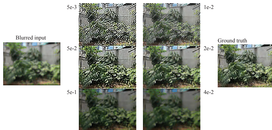
FIGURE 7.11: Left shows an image blurred with a gaussian, \sigma = 3 ; center left shows regularized least squares reconstructions for different values of the regularization constant; center right shows deblurred images, using the TVD strategy of Section ??; and right shows the ground truth image (more details in the caption of Figure 7.8). TVD has a much harder time controlling these components than for Figure 7.10. Image credit: Figure shows my photograph of a delicious monster in Sao Paulo.
