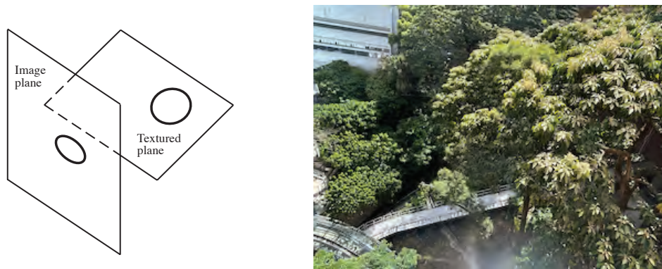
FIGURE 19.3: On the left an example of foreshortening. A circle on a world plane looks like an ellipse in an image plane, because the world plane is tilted backwards. Try this by holding your hand in front of your face, then tilting it backward – it gets shorter in the tilted dimension. If you knew that you were viewing a plane covered in circles, the shape of the texture elements in the image would give you a cue to the orientation of the plane. Some version of this cue seems to be used by people. On the right , an image of trees at HKU. Notice how the leaves on each tree seem to give you a cue to the shape of its surface. Elementary methods for exploiting this cue are both intricate and obsolescent, but the cue is powerful. Image credit: My photograph of trees at HKU.
