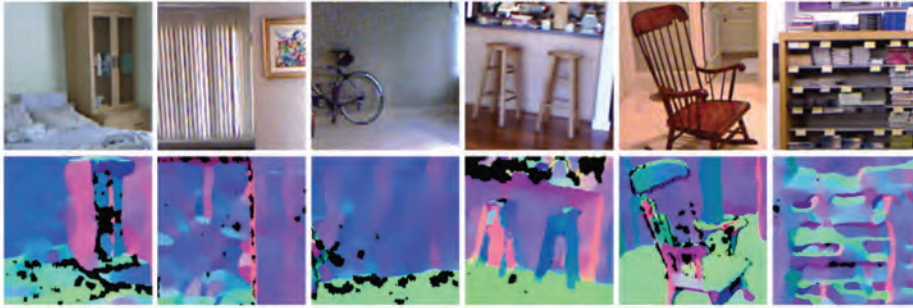
FIGURE 19.7: Ground truth normals estimated from depth measurements can present difficulties. The top row shows images from the NYUV2 dataset of Figure 19.7. Bottom row shows normal estimates derived from the depth, and used as ground truth on occasion. Normal estimates are rendered by mapping R, G and B to components of the normal. Here, a normal pointing to the left in the image is pink, one pointing up in the image is light green, and the normal of a frontal surface is blue. These estimates aren't the same as the true normals (look at the venetian blinds, for example; the blodges on the back wall in the bicycle image or the bedroom image; and the blodges in the bookshelf image). Evidence that the difficulty comes from problem depth predictions includes the tendency of deformations to start at surface boundaries and to be concentrated at shadow effects. Image credit: Figure 2 of “Estimating and Exploiting the Aleatoric Uncertainty in Surface Normal Estimation” Gwangbin Bae Ignas Budvytis Roberto Cipolla
