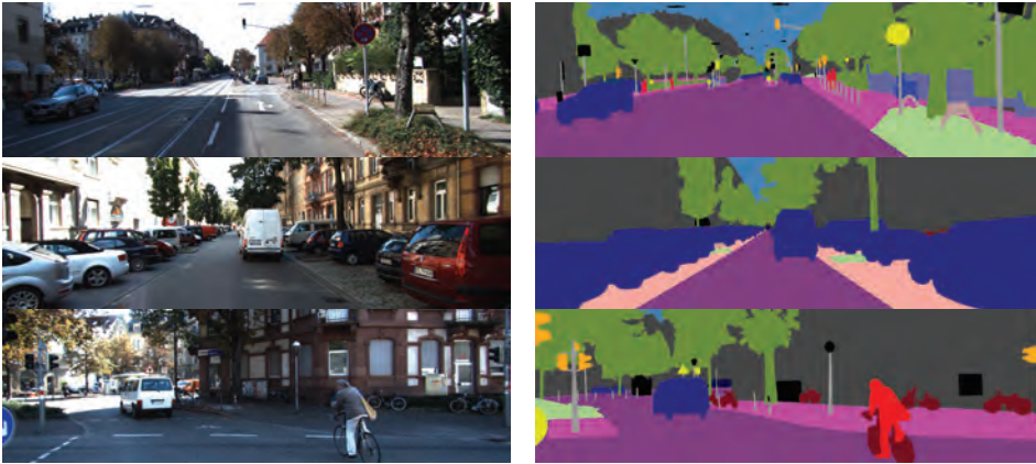
FIGURE 21.1: Semantic segmentation places a label taken from some taxonomy at each pixel in an image. On the left, three example images from a well-known dataset for semantic segmentation (KITTI). On the right, semantic segmentations of each image from the ground truth. The color at each location corresponds to the label (deep purple for roads, blue for cars, bright red for people, and so on).
