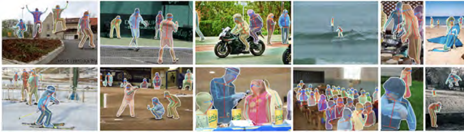
FIGURE 25.8: The feature produced by ROIAlign can be decoded into a range of useful predictions. This figure shows masks predicted for humans. On top of the masks are predicted locations for keypoints (points on the body, typically at joints). These are obtained by passing the ROIAlign feature through a convolutional network and interpreting the resulting data block as keypoint locations. Image Credit: Part of Figure 5 of Mask R-CNN Kaiming He Georgia Gkioxari Piotr Dollár Ross Girshick
