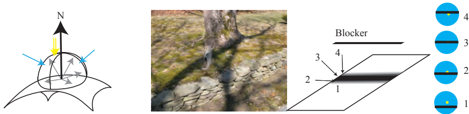
FIGURE 29.4: Some outdoor shadows have blurred outlines, because the sun occupies a small range of directions in the sky – when you look up, it looks like a small circle not a point. On the left, a point on a diffuse surface receives light from the sun (yellow arrows) and from the sky (blue arrows) and reflects this light evenly spread around all outgoing directions. The image is a picture by Pamela V White, published on Flickr with a creative commons license ( https://creativecommons.org/licenses/by-sa/2.0/ ). On the center right, a blocker stopping the ground from seeing the sun. The sun is quite high in the sky, and the blocker is high off the ground, meaning it blocks a small range of directions. At 1, the surface can see the whole of the sun. At 2 and 4, the surface can see only part of the sun because the blocker covers part of it. At 3, the blocker covers all of the sun.
