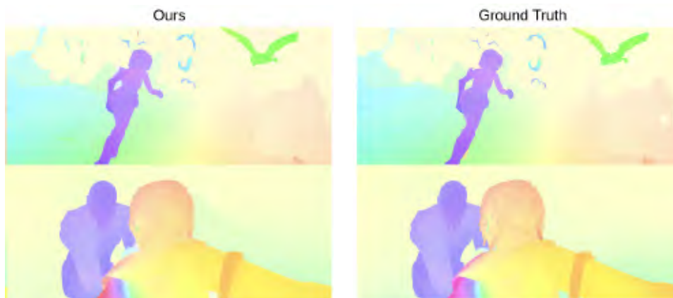
FIGURE 34.16: Flow fields predicted by RAFT are very close to ground truth when it is available. Strong discontinuities in flow generate no noticeable difficulties. These flow fields are obtained from two frames from the SINTTEL dataset ( left ), compared with ground truth ( right ). SINTTEL is a dataset of rendered frames from a CGI movie, so the true flow can be known. The direction of a flow vector is shown by hue (what changes from red to yellow to green to purple) and the magnitude by saturation (very small vectors are white, longer are pale colors, longest have intense colors). Image credit: Figure 1 of RAFT: Recurrent All-Pairs Field Transforms for Optical Flow by Z. Teed and J. Deng.
