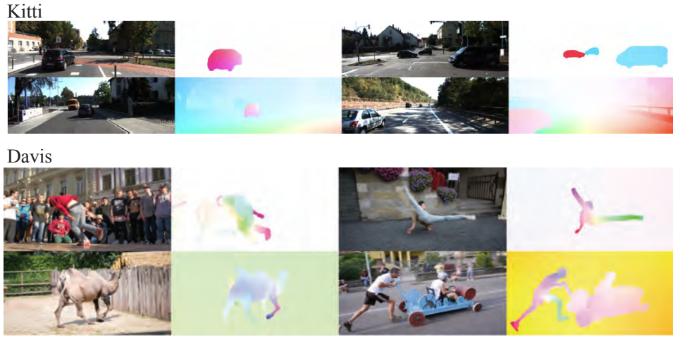
FIGURE 34.17: For real images, there is no ground truth to compare to. This figure shows flow fields predicted by RAFT for two datasets. KITTI data has to do with autonomous vehicles. The DAVIS dataset is at 1088 \times 1920 resolution. Flow fields should look plausible to you (for example, low flow at distant objects; strong discontinuities in flow around object boundaries). Image credit: Figure 1 of RAFT: Recurrent All-Pairs Field Transforms for Optical Flow by Z. Teed and J. Deng.
