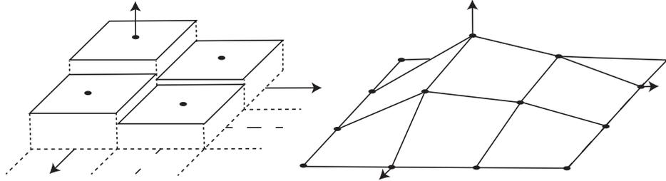
FIGURE 3.1: On the **left**, a function interpolating a  $2 \times 2$  image using nearest neighbors. The dashed lines pass through grid points, and the dotted lines are halfway between grid points. The function is zero from the four boxes shown. Image values are shown as filled circles. On the **right**, a bilinear interpolate of the same data.
