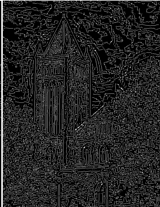
low threshold (weak edges)
