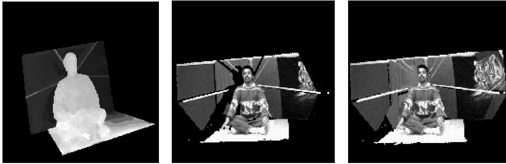
Figure 26.6 Multicamera stereo. From left to right: the range map associated with a cluster of cameras; a texture-mapped image of the corresponding mesh, observed from a different viewpoint; note the dark areas associated with depth discontinuities in the map; a texture-mapped image constructed from two adjacent camera clusters; note that the gaps have been filled. Reprinted from “Virtualized Reality: Constructing Virtual Worlds From Real Scenes,” by T. Kanade, P.W. Rander and J.P. Narayanan, IEEE Multimedia , 4(1):34–47, (1997). © 1997 IEEE.
