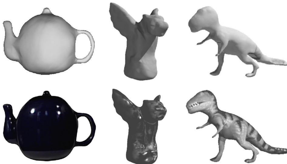
Figure 26.5 Shaded and texture-mapped models of a teapot, gargoyle and dinosaur. The teapot was constructed from six registered photographs; the gargoyle and dinosaur models were each built from nine images. Reprinted from “Automatic Model Construction, Pose Estimation, and Object Recognition from Photographs Using Triangular Splines,” by S. Sullivan and J. Ponce, IEEE Transactions on Pattern Analysis and Machine Intelligence, 20(10):1091–1096, (1998). © 1998 IEEE.
