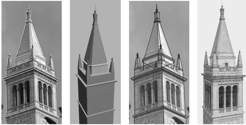
Figure 26.8 Façade model of the Berkeley Campanile. From left to right: A photograph of the Campanile, with selected edges overlaid; the 3D model recovered by photogrammetric modeling; reprojection of the model into the photograph; a texture-mapped view of the model. Reprinted from “Modeling and Rendering Architecture from Photographs: A Hybrid Geometry- and Image-Based Approach,” by P. Debevec, C.J. Taylor, and J. Malik, Proc. SIGGRAPH , (1996). © 1996 ACM, Inc. Included here by permission.
