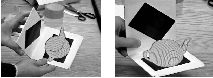
Figure 26.10 Augmented reality experiment. The (affine) world coordinate system is defined by corners of the black polygons. Reprinted from “Calibration-Free Augmented Reality,” by K. Kutulakos and J. Vallino, IEEE Transactions on Visualization and Computer Graphics , 4(1):1–20, (1998). © 1998 IEEE.
