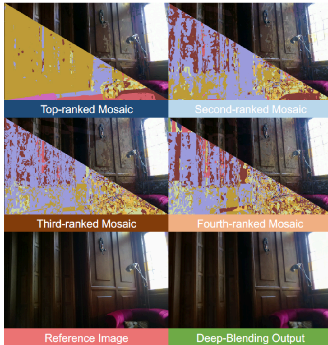
Fig. 10. Our network takes as input ranked mosaics generated from a set of warped candidate views. For each pixel, the candidates are ranked based on their expected blending contribution, and 4 color-image mosaics are formed from the top 4 rankings. Example mosaics are shown in the first two rows. The top right halves show the color mosaic, while the bottom left halves show colormaps of the selection, with each input shown in a different color. Weighted blending outputs from our network (bottom right) are trained by minimizing their difference with real images (bottom left). Our network also blends an RGB view of the global mesh (not shown).
