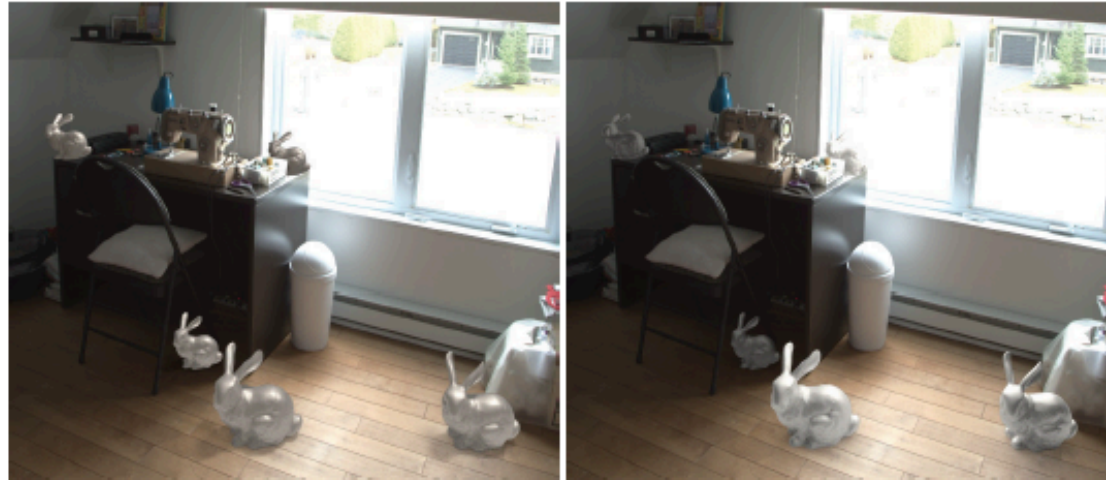
Figure 1. Indoor lighting is spatially-varying. Methods that estimate global lighting [8] (left) do not account for local lighting effects resulting in inconsistent renders when lighting virtual objects. In contrast, our method (right) produces spatially-varying lighting from a single RGB image, resulting in much more realistic results.
