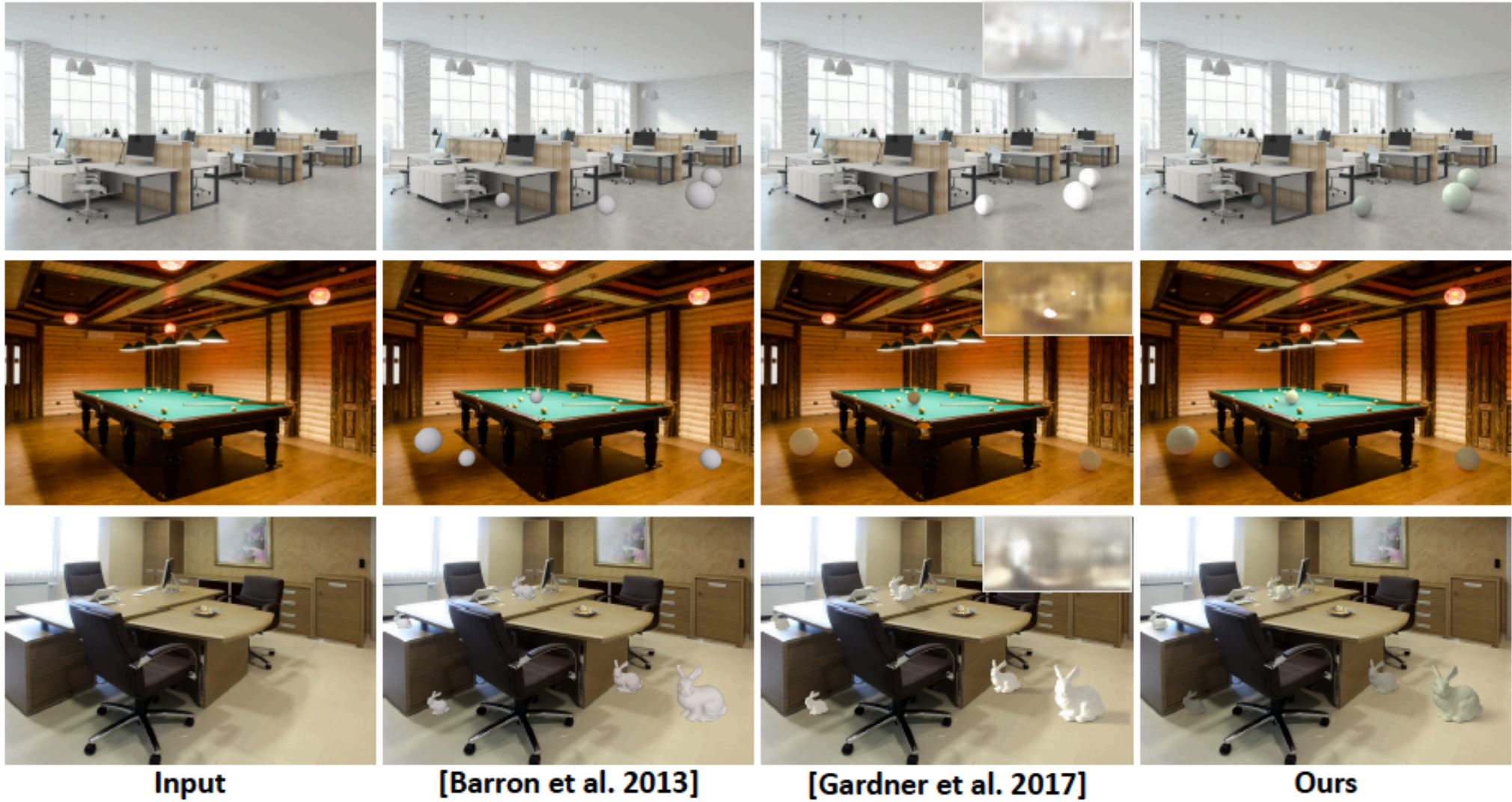
Figure 14. Object insertion examples and comparisons. Our proposed method estimates shape (depth and surface normals), spatially-varying, complex reflectance (based on a micro-facet SVBRDF model) and spatially-varying lighting from a single image of an indoor scene. Given these estimates, we can insert virtual 3D objects into these images and produce photo-realistic results where the objects look like they truly belong in the scene. Note the shading and specular highlights on the inserted spheres, the realistic shadows cast on the ground, the reflection from the ground onto the spheres and adaptation of the appearance of the spheres to the local shadows and shading in the scene. We also compare with previous works of Barron et al. [6] and Gardner et al. [20] on real images. Note that in the results of [20], the shadows of some objects might be truncated by the plane we segment from the scene.
