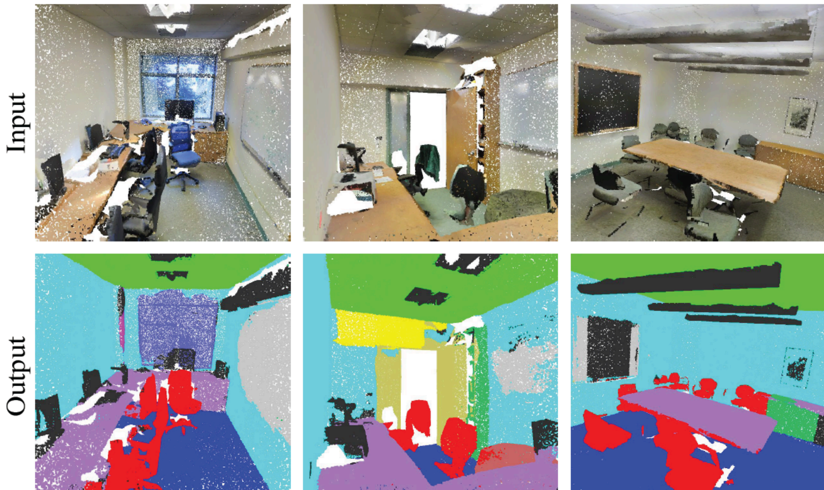
Figure 4. Qualitative results for semantic segmentation. Top row is input point cloud with color. Bottom row is output semantic segmentation result (on points) displayed in the same camera viewpoint as input.
