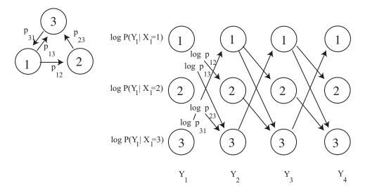
FIGURE 9.7: At the top left, a simple state transition model. Each outgoing edge has some probability, though the topology of the model forces two of these probabilities to be 1. Below, the trellis corresponding to that model. Each path through the trellis corresponds to a legal sequence of states, for a sequence of three measurements. We weight the arcs with the log of the transition probabilities, and the nodes with the log of the emission probabilities. I have shown some weights
