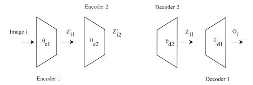
Two layers of denoising auto-encoder, ready for fine tuning. This FIGURE 14.3: figure should help with the notation in the text.
