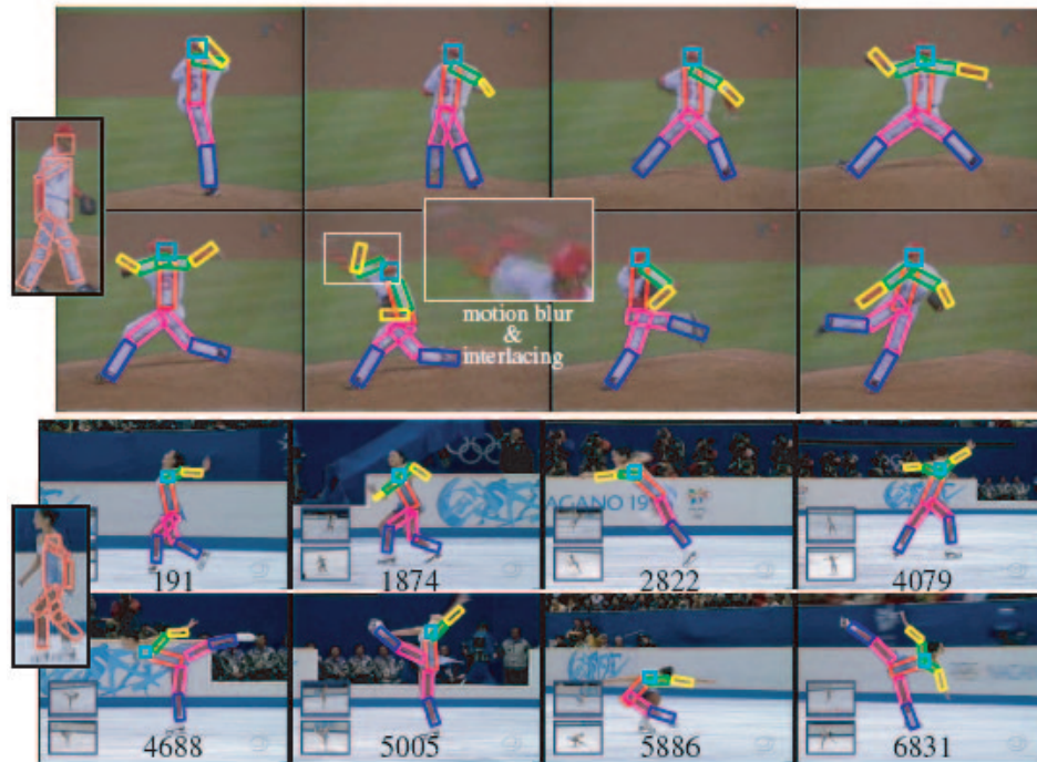
Figure 3.12: Deva's thesis Frames from sequences tracked with the methods of Ramanan et al., where a discriminative appearance model is built using a specialized detector (figure ), and then detected in each frame using a pictorial structures model. The figure shows commercial sports footage with fast and extreme motions. On the top , results from a 300 frame sequence of a baseball pitch from the 2002 World Series. On the bottom , results from the complete medal-winning performance of Michelle Kwan from the 1998 Winter Olympics. We label frame numbers from the 7600-frame sequence. For each sequence, the system first runs a walking pose finder on each frame, and uses the single frame with the best score (shown in the left insets ) to train the discriminative appearance models. In the baseball sequence, the system is able to track through frames with excessive motion blur and interlacing effects (the center inset ). In the skating sequence, the system is able to track through extreme poses for thousands of frames. The process is fully automatic.
