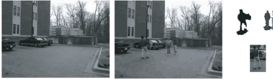
Fig. 2.1 Fig 1 of surveillance/00868683 Background subtraction identifies groups of pixels that differ significantly from a background model. The method is most useful for some some cases of surveillance, where one is guaranteed a fixed viewpoint and a static background changing slowly in appearance. On the left , a background model; in the center , a frame; and on the right , the resulting image blobs. The figure is taken from Haritaoglu et al. [168]; in this paper, authors use an elaborate method involving a combination of thresholds to obtain good blobs. Figure 2.2 illustrates a method due to these authors that obtains a kinematic configuration estimate by parsing the blob. Figure from “W4: Real-time surveillance of people and their activities”, Haritaoglu et al. , IEEE Trans. Pattern Analysis and Machine Intelligence, 2000, © 2000 IEEE
