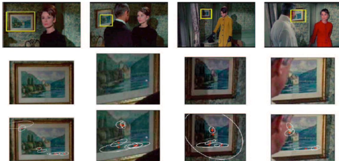
FIGURE 16.7: This figure shows results from the query of Figure 16.5, obtained by looking for image regions that have a set of visual words strongly similar to those found in the query region. The first row shows the whole frame from the video sequence; the second row shows a close-up of the box that is the result (indicated in the first row); and the third row shows the neighborhoods in that box that generated visual words that match those in the query. Notice that some, but not all, of the neighborhoods in the query were matched. This figure was originally published as Figure 11 of J. Sivic and A. Zisserman "Efficient Visual Search for Objects in Videos," Proc. IEEE, Vol. 96, No. 4, April 2008 © IEEE 2008.
