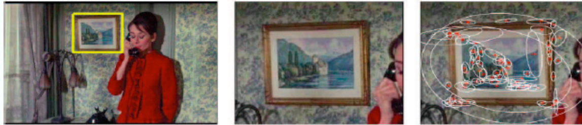
FIGURE 16.5: The original application of visual word representations was to search video sequences for particular patterns. On the left, a user has drawn a box around a pattern of interest in a frame of video; the center shows a close-up of the box. On the right, we see neighborhoods computed from this box. These neighborhoods are ellipses, rather than circles; this means that they are covariant under affine transforms. Equivalently, the neighborhood constructed for an affine transformed patch image will be the affine transform of the neighborhood constructed for the original patch (definition in Section 5.3.2). This figure was originally published as Figure 11 of J. Sivic and A. Zisserman "Efficient Visual Search for Objects in Videos," Proc. IEEE, Vol. 96, No. 4, April 2008 © IEEE 2008.
