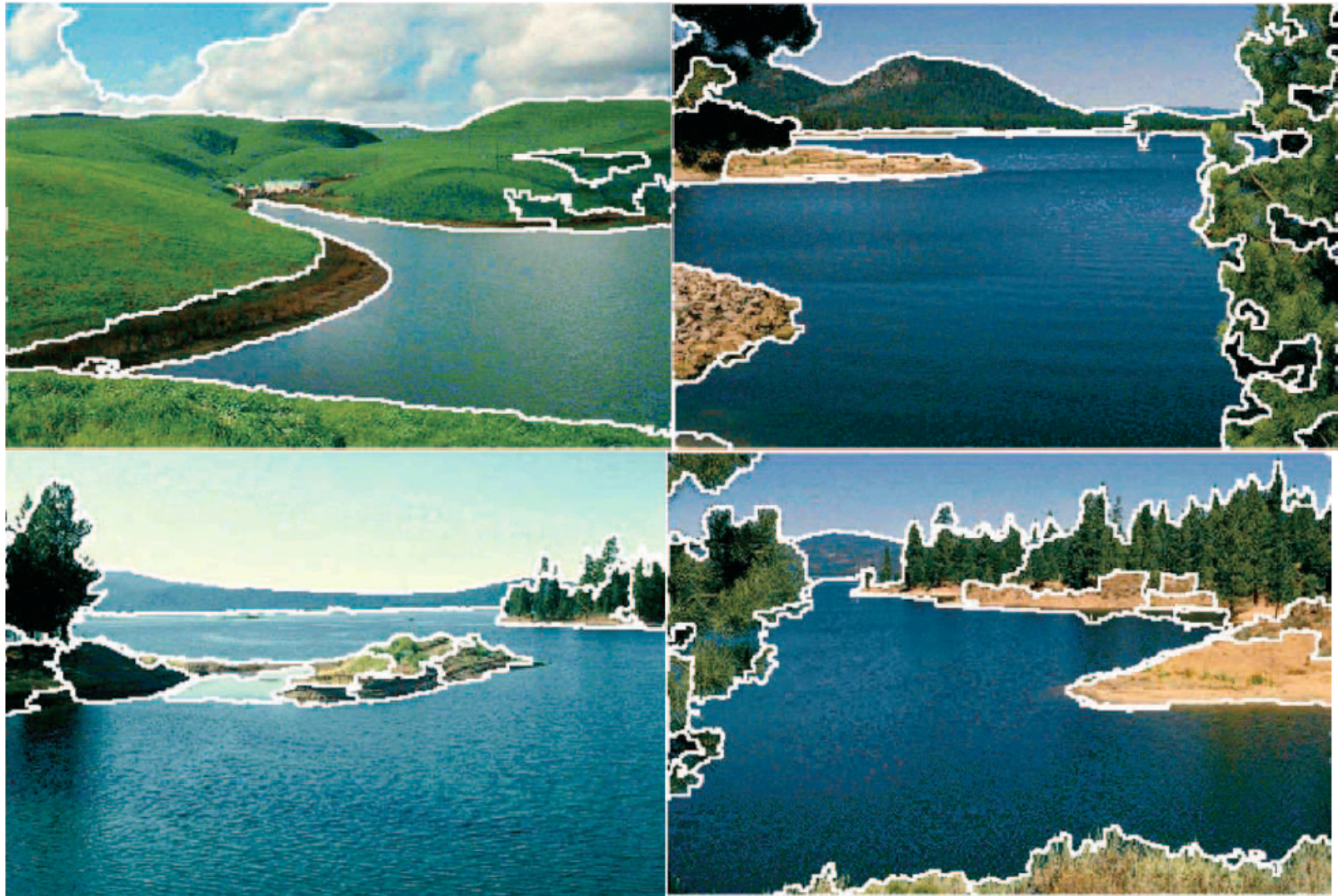
FIGURE 9.21: Segmentations of images obtained using the mean shift algorithm. This figure was originally published as Figure 10 of “Mean Shift: A Robust Approach Toward Feature Space Analysis,” by D. Comaniciu and P. Meer, IEEE Transactions on Pattern Analysis and Machine Intelligence, 2002 © IEEE, 2002.
