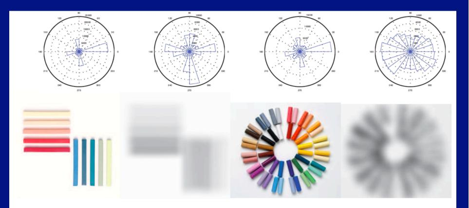
FIGURE 5.9: Different patterns have quite different orientation histograms. The left shows rose plots and images for a picture of artists pastels at two different scales; the **right** shows rose plots and images for a set of pastels arranged into a circular pattern. Notice how the pattern of orientations at a particular scale, and also the changes across scales, are quite different for these two very different patterns. *Philip Gatward* © *Dorling Kindersley, used with permission.*
