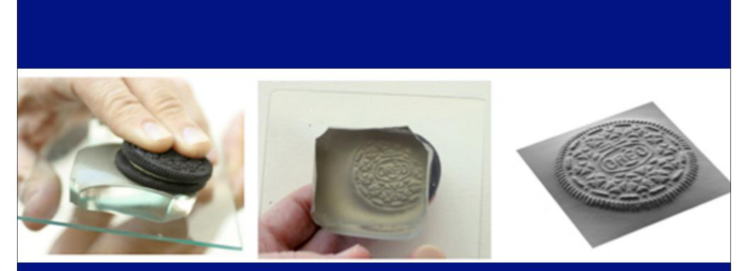
M.K. Johnson and E.H. Adelson "Retrographic sensing for the measurement of surface texture and shape" CVPR, 2009
