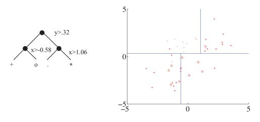
FIGURE 3.5: A straightforward decision tree, illustrated in two ways. On the left, I have given the rules at each split; on the right, I have shown the data points in two dimensions, and the structure that the tree produces in the feature space.
