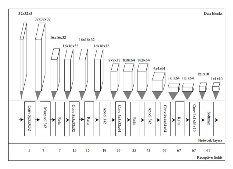
Figure 17.15: Three different representations of the simple network used to classify CIFAR-10 images for this example. Details in the text
