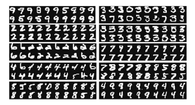
Figure 17.11: Visualizing the patterns that the final stage ReLUs respond to for the simple CIFAR example. Each block of images shows the images that get the largest output for each of 10 ReLUs (the ReLUs were chosen at random from the 500 available). Notice that these ReLU outputs don't correspond to class—these outputs go through a fully connected layer before classification—but each ReLU clearly responds to a pattern, and different ReLUs respond more strongly to different patterns
