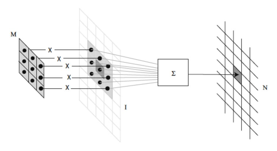
Figure 17.4: To compute the value of N at some location, you shift a copy of M to lie over that location in I; you multiply together the non-zero elements of M and I that lie on top of one another; and you sum the results
