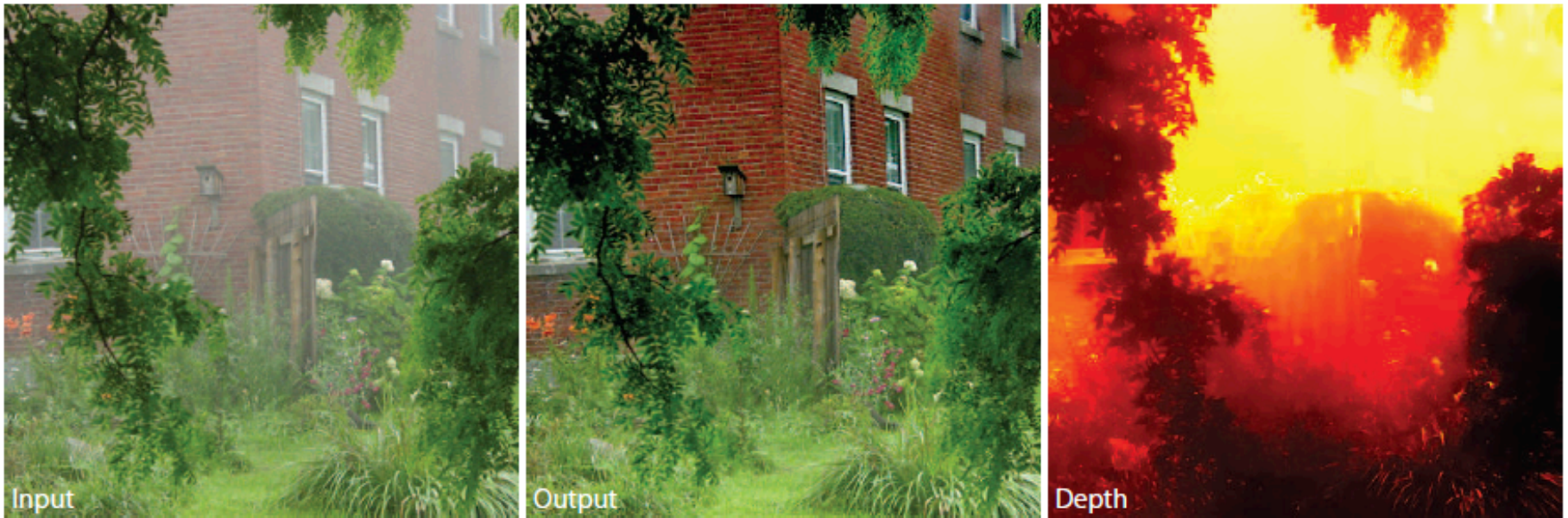
Figure 1: Dehazing based on a single input image and the corresponding depth estimate.
