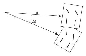
$$\left[ \begin{array}{c} x \\ y \\ \theta \end{array} \right] \rightarrow \left[ \begin{array}{c} x + R(\sin(\theta + \Delta\theta) - \sin\theta) \\ y - R(\cos(\theta + \Delta\theta) - \cos\theta) \\ \theta + \Delta\theta \end{array} \right]$$
