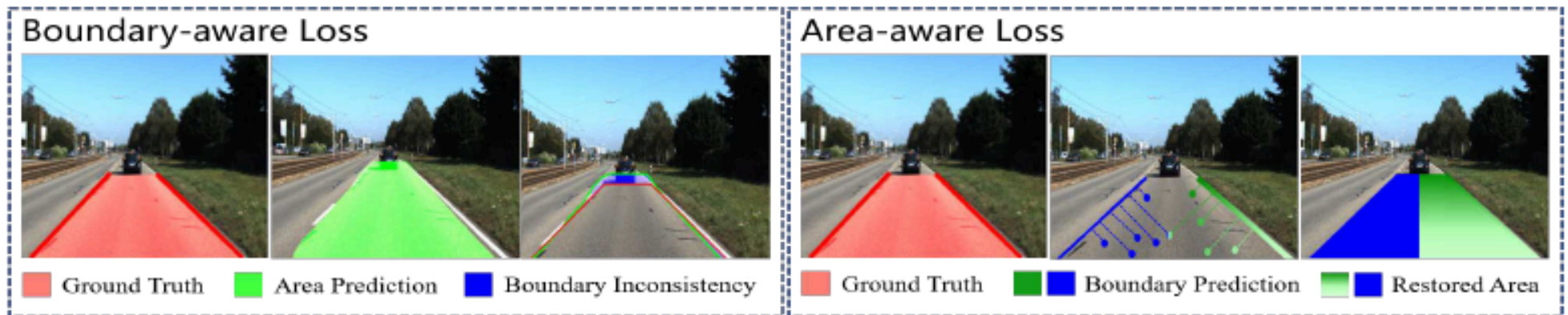
Fig. 5. Boundary-aware loss and area-aware loss. Left: An illustration of our boundary-aware loss. The blue area indicates boundary inconsistency. Right: An illustration of our area-aware loss. Different intensities in prediction areas indicate different prediction confidence. The difference between restored area and ground truth indicates the area aware loss.
