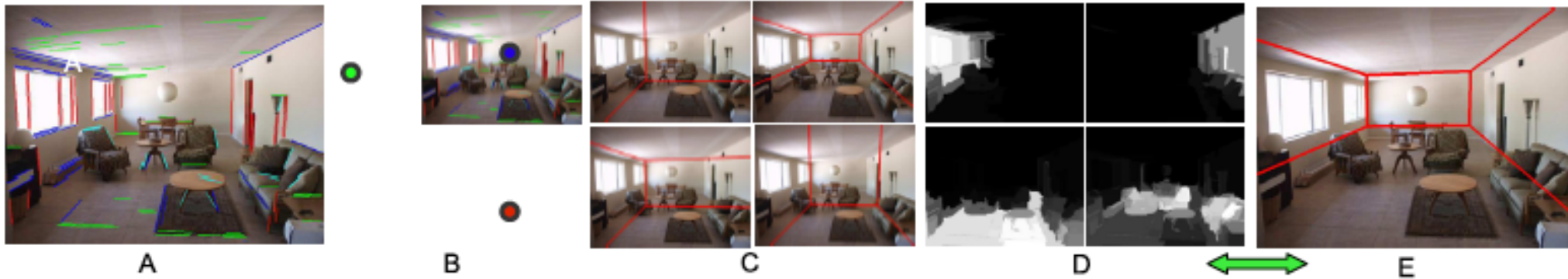
Figure 2. Our process takes the original image, identifies long line segments (A), and uses these to find vanishing points (B). The line segments in (A) are colored with the color of the vanishing point they vote for. This information, and other features, are used to produce a set of possible layouts, which are ranked by a function learned with structure learning (four are shown in C). The top ranked layouts produce maps of label probabilities (shown in D for “left wall”, “floor”, “right wall” and “object”). In turn these maps are used to re-estimate features, and the re-estimated features are used to produce a second ranking. The top ranked layout for this image is in (E).
