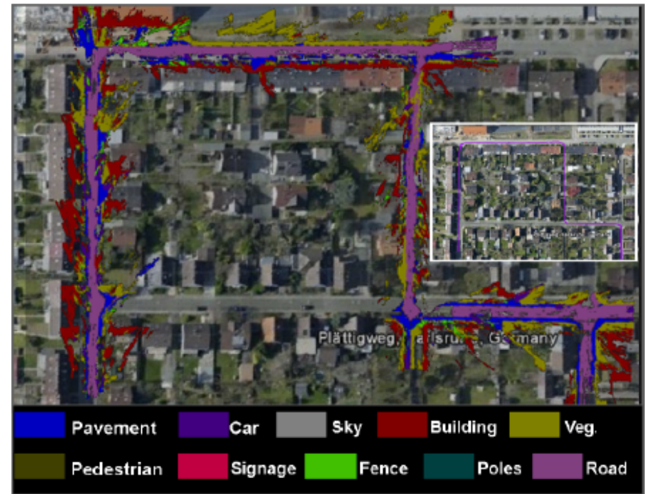
Fig. 8: Semantic model of the reconstructed scene overlaid with the corresponding Google Earth image. The inset image shows the Google earth track of the vehicle.
