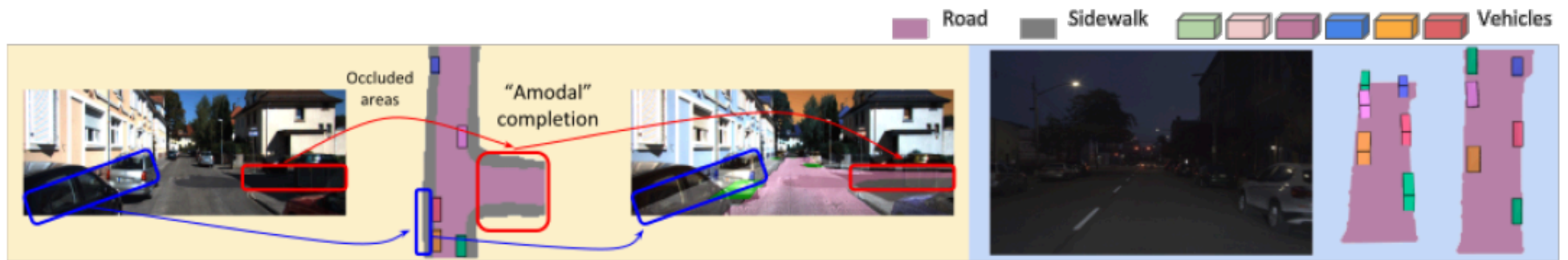
Figure 1: MonoLayout : Given only a single image of a road scene, we propose a neural network architecture that reasons about the amodal scene layout in bird’s eye view in real-time (30 fps). Our approach, dubbed MonoLayout can hallucinate regions of the static scene (road, sidewalks)—and traffic participants—that do not even project to the visible regime of the image plane. Shown above are example images from the KITTI [10] (left) and Argoverse [5] (right) datasets. MonoLayout outperforms prior art (by more than a 20% margin) on hallucinating occluded regions.
