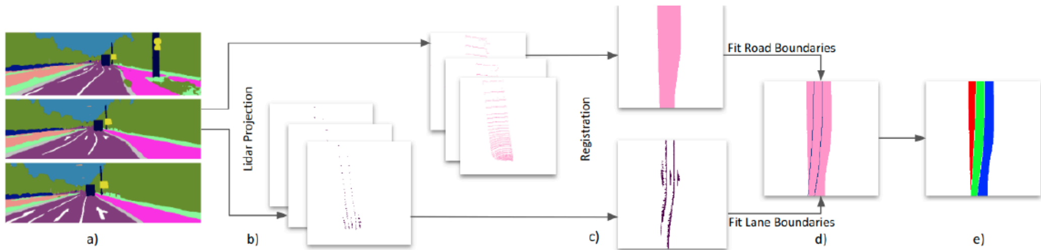
Fig. 3: Weak Supervision setup: We show our automated (noisy) label generation scheme herein. Points from the lidar frame are projected down to semantically segmented images (a), to obtain sparse static layouts (b). These sparse layouts are stacked across an image sequence to generate dense static layouts (c). In the next step (d), road and lane boundaries are extracted and combined to obtain lane layouts (e).
