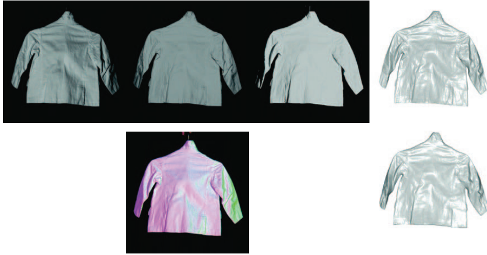
FIGURE 4.6: Photometric stereo could become the method of choice to capture complex deformable surfaces. On the top , three images of a garment, lit from different directions, which produce the reconstruction shown on the top right . A natural way to obtain three different images at the same time is to use a color camera; if one has a red light, a green light, and a blue light, then a single color image frame can be treated as three images under three separate lights. On the bottom , an image of the garment captured in this way, which results in the photometric stereo reconstruction on the bottom right .
