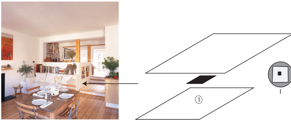
FIGURE 2.10: The photograph on the left shows a room interior. Notice the lighting has some directional component (the vertical face indicated by the arrow is dark, because it does not face the main direction of lighting), but there are few visible shadows (for example, the chairs do not cast a shadow on the floor). On the right , a drawing to show why; here there is a small occluder and a large area source. The occluder is some way away from the shaded surface. Generally, at points on the shaded surface the incoming hemisphere looks like that at point 1. The occluder blocks out some small percentage of the area source, but the amount of light lost is too small to notice (compare figure 2.9). Jake Fitzjones © Dorling Kindersley, used with permission.
