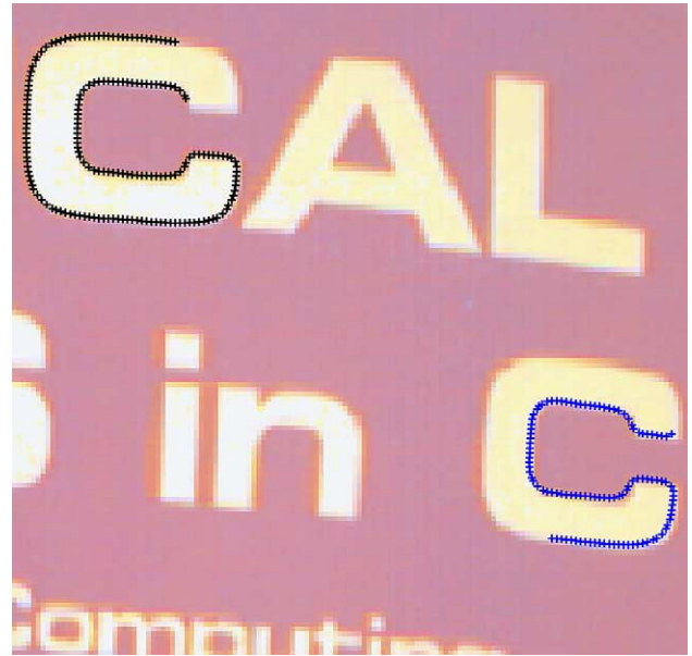
Fig. 1. 2D curves to be registered. The curves are subsets of the output of an edge detector applied to the image. Synthetic rotations and translations of the lower-right 'C' are registered to the upper left one.
