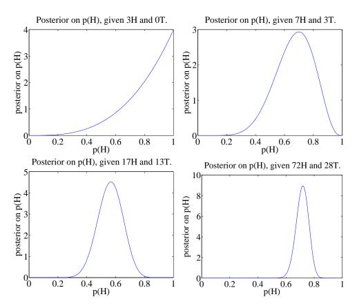
FIGURE 8.2: The probability that an unknown coin will come up heads when flipped is p(H). For these figures, I simulated coin flips from a coin with p = 0.75. I then plotted the posterior for various data. Notice how, as we see more flips, we get more confident about p. The vertical axis changes substantially between plots in this figure.
