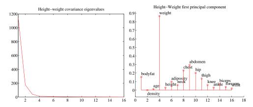
FIGURE 10.29: On the left, the eigenvalues of the covariance matrix for the bodyfat data set. Notice how fast the eigenvalues fall off; this means that most principal components have very small variance, so that data can be represented well with a small number of principal components. On the right, the first principal component for this dataset, plotted using the same convention as for figure 10.28.
