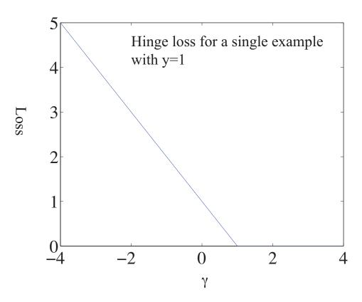
FIGURE 11.1: The hinge loss, plotted for the case  $y_i = 1$ . The horizontal variable is the  $\gamma_i = \mathbf{a} \cdot \mathbf{x}_i + b$  of the text. Notice that giving a strong negative response to this positive example causes a loss that grows linearly as the magnitude of the response grows. Notice also that giving an insufficiently positive response also causes a loss. Giving a strongly positive response is free.
