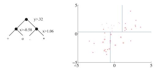
FIGURE 11.5: A straightforward decision tree, illustrated in two ways. On the left, I have given the rules at each split; on the right, I have shown the data points in two dimensions, and the structure that the tree produces in the feature space.
