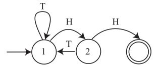
FIGURE 7.1: A finite state machine representing the coin flip example. By convention, the end state is a double circle, and the start state has an incoming arrow. I've labelled the arrows with the event that leads to the transition, but haven't bothered to put in the probabilities, because each is 0.5.
