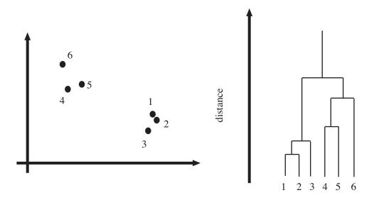
FIGURE 12.1: Left, a data set; right, a dendrogram obtained by applomerative clustering using single-link clustering. If one selects a particular value of distance, then a horizontal line at that distance splits the dendrogram into clusters. This representation makes it possible to guess how many clusters there are and to get some insight into how good the clusters are.
