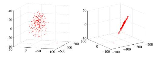
FIGURE 10.26: Two views of a multidimensional scaling to three dimensions of the height-weight dataset. Notice how the data seems to lie in a flat structure in 3D, with one outlying data point. This means that the distances between data points can be (largely) explained by a 2D representation.
