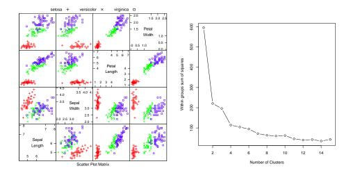
FIGURE 12.11: On the left, the scatterplot matrix for the Iris data, for reference. On the right, a plot of the value of the cost function for each of several different values of k. Notice how there is a sharp drop in cost going from k=1 to k=2, and again at k = 4; after that, the cost falls off slowly. This suggests using k = 2, k=3, or k=4, depending on the precise application.
