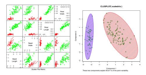
FIGURE 12.8: On the left, a panel plot of the iris data clustered using k-means with k=2. By comparison with figure 12.11, notice how the versicolor and verginica clusters appear to have been merged. On the right, this data set projected onto the first two principal components, with one blob drawn over each cluster.
