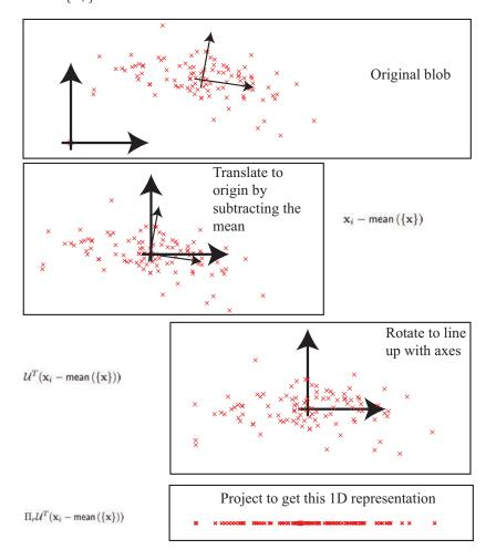
FIGURE 10.15: Computing a low dimensional representation for principal components analysis.
