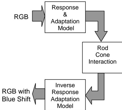
**Figure 2: Block Diagram of our Blue Shift Operator.** The response and adaptation model creates retina like rod responses to the input image. These rod responses are fed into the rod-cone interaction operator which calculates the cone responses. Finally using the cone responses we determine the hue of the blue shift image.
