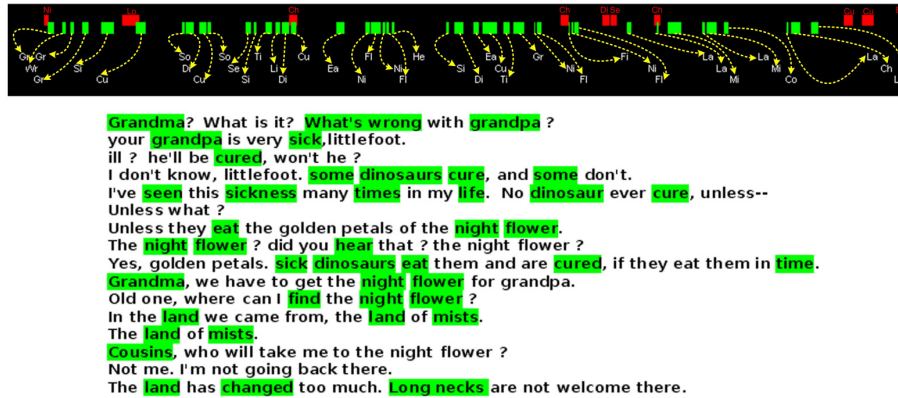
Figure 6. Top: A timeline for a second block, with discriminative word model responses marked. The green blocks represent correct detections, the red blocks represent false positives. We are not aware of false negatives. Each green block is linked to the first letter of the word it represents in the transcript below (where spotted words are marked in green). Figure 5 shows another such sequence.
