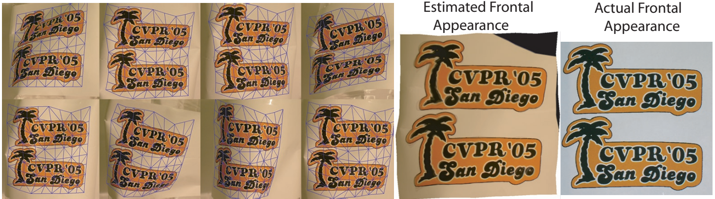
Figure 6: We automatically compute the frontal appearance of a deforming surface — allowing us to compute normals and thus estimate shape (figure 7). The estimated frontal texture is an average of the eight images, each pushed through the appropriate warping. We require the user to manually select the four corners of the texture in a single view (in this case, the upper right image). Then we automatically deform this model to find matches in each of the other frames (a total of eight in this case). The blue mesh in each of the images on the left indicates the match. Following the method outlined in the text, we compute estimated frontal edge lengths, then, treating these lengths as rest-lengths for springs, we minimize energy. Without assuming any form of surface rigidity, this method requires three views of the deforming surface. However, because of degeneracies that arise in practice, we use eight. Degenerate triangles occur when there is a single axis of rotation between views — detecting these degeneracies is described in section 5.1.
