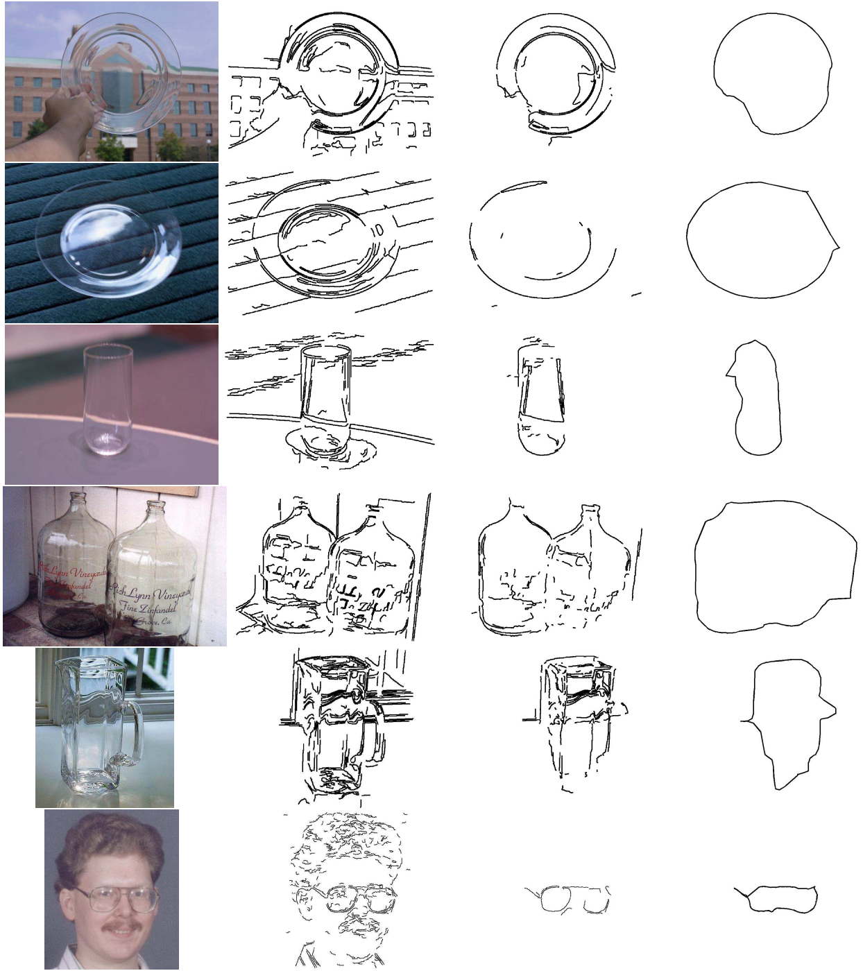
Figure 7: Test images and output from the described system. Left: Six sample test images, Middle left: Edges from edge detector, Middle right: Edges that have been labeled as glass. Right: Regions of glass found by shrinking a snake around the labeled glass edges.
