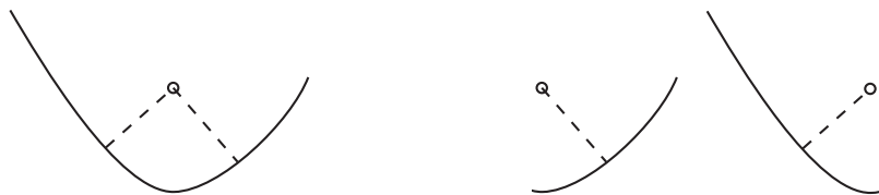
FIGURE 12.3: There can be more than one point on a curve that looks as if it is closest to a token. This makes fitting curves to points very difficult. On the left , a curve and a token; dashed lines connect the token to the two points on the curve that could be closest. The dashed line from token to curve and the tangent to the curve are at right angles for each of the two points on the curve. Center and right show copies of part of the curve; for each, the closest point on the segment to the token is different, because part of the curve is missing. As a result, no local test can guarantee a point is closest – all candidates must be checked.
