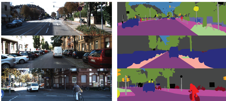
FIGURE 22.7: Semantic segmentation places a label taken from some taxonomy at each pixel in an image. On the left, three example images from a well-known dataset for semantic segmentation (KITTI). On the right, semantic segmentations of each image from the ground truth. The color at each location corresponds to the label (deep purple for roads, blue for cars, bright red for people, and so on).
