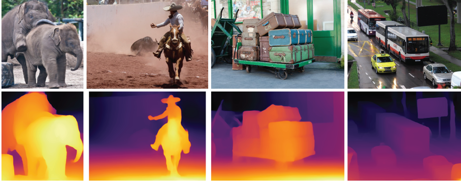
FIGURE 19.5: Predicting depth from single images is now a reliable technology. Top row shows images; bottom row , predicted depth representations. The predictor reports a_d\delta + b_d where \delta is disparity and a_d, b_d are per image constants. Orange is closer to the eye, purple is further from the eye. Notice: depth maps contain quite fine detail (eg the larger elephant’s trunk; where the rider contacts the horse; the grooves between suitcases); small depth gradients are well represented (eg along the cowboy’s arm); windows can cause confusion (eg window next to suitcases). Image credit: Figure 1 of “Towards Robust Monocular Depth Estimation: Mixing Datasets for Zero-shot Cross-dataset Transfer”, René Ranftl*, Katrin Lasinger*, David Hafner, Konrad Schindler, and Vladlen Koltun.
