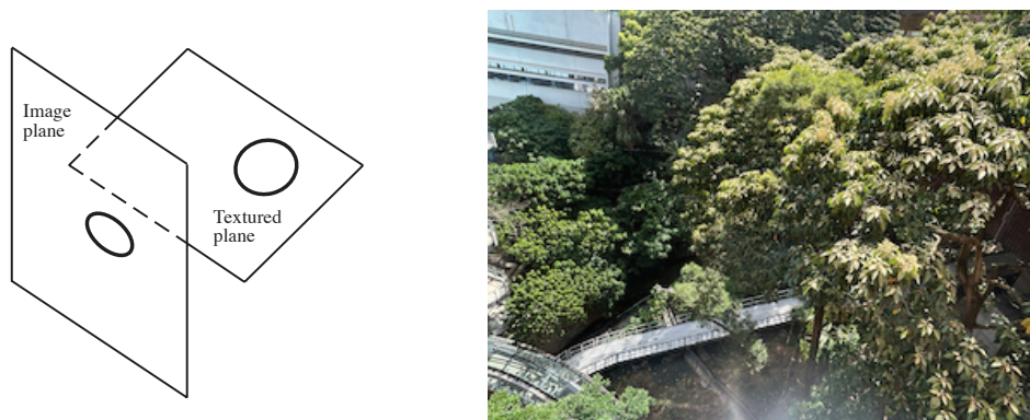
FIGURE 19.7: On the left an example of foreshortening. A circle on a world plane looks like an ellipse in an image plane, because the world plane is tilted backwards. Try this by holding your hand in front of your face, then tilting it backward – it gets shorter in the tilted dimension. If you knew that you were viewing a plane covered in circles, the shape of the texture elements in the image would give you a cue to the orientation of the plane. Some version of this cue seems to be used by people. On the right , an image of trees at HKU. Notice how the leaves on each tree seem to give you a cue to the shape of its surface. Elementary methods for exploiting this cue are both intricate and obsolescent, but the cue is powerful. Image credit: My photograph of trees at HKU.
