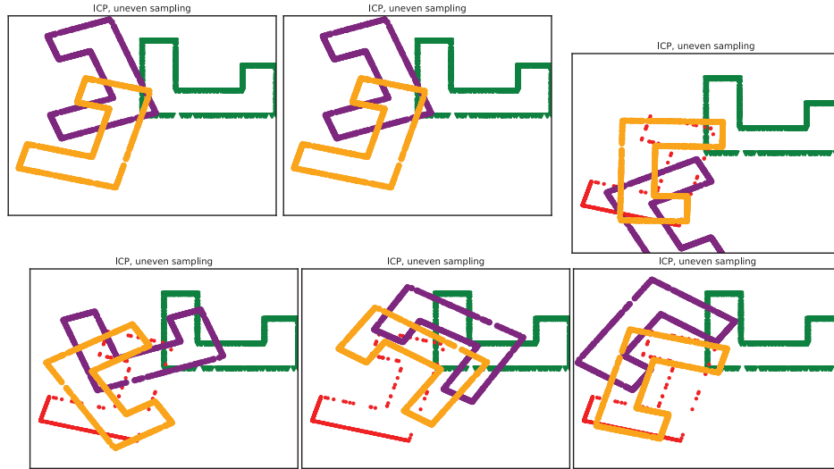
FIGURE 14.8: If the two shapes that have been sampled differently, ICP can produce poor results. The green (upward pointing, to the right) u shape must be transformed to lie on the red (sideways pointing, to the left) u shape. The initial transformation is shown by the purple shape. The ICP result is shown in orange . The two offset cases are successful; the others are not.
