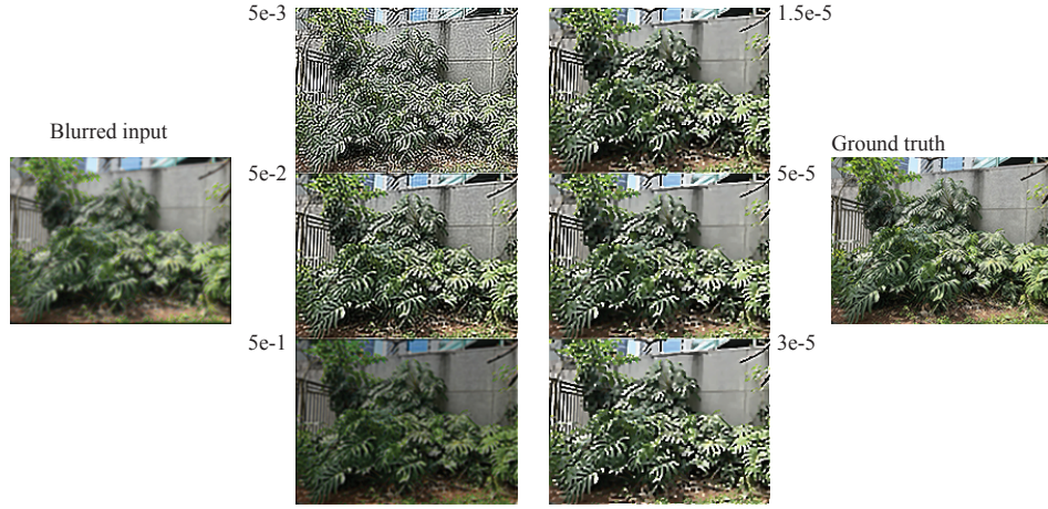
FIGURE 7.7: Left shows an image blurred with a gaussian, \sigma = 1 ; center left shows regularized least squares reconstructions for different values of the regularization constant; center right shows deblurred images, using the WLS strategy of Section ??; and right shows the ground truth image. Notice that there must be many very small eigenvalues in \mathcal{B} , because when the regularization constant is small, the reconstruction is almost unrecognizable (the black and white “snakeskin” pattern is a set of very high frequency components that are easily smoothed out – which is why they correspond to small eigenvalues). Increasing the regularization constant helps control these patterns, but increasingly darkens the reconstruction. The WLS method requires an estimate of the gradient, which I took from the least-squares reconstruction. WLS helps control these components, but the best reconstruction certainly isn’t perfect. Scoring whether a reconstruction is “like” an image is difficult. Image credit: Figure shows my photograph of a delicious monster in Sao Paulo.
