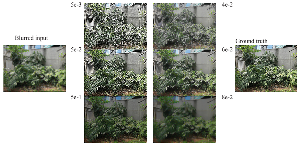
FIGURE 7.9: Left shows an image blurred with a gaussian, \sigma = 1 ; center left shows regularized least squares reconstructions for different values of the regularization constant; center right shows deblurred images, using the TVD strategy of Section ??; and right shows the ground truth image (more details in the caption of Figure 7.7). TVD can control the problem high frequency components, with an appropriate choice of weight. Image credit: Figure shows my photograph of a delicious monster in Sao Paulo.
