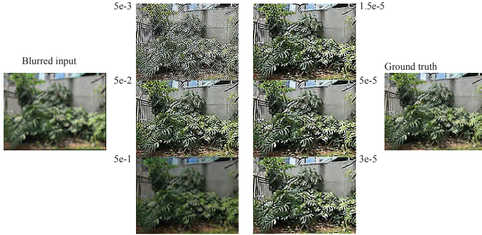
FIGURE 7.8: Left shows an image blurred with a gaussian, \sigma = 1 ; center left shows regularized least squares reconstructions for different values of the regularization constant; center right shows deblurred images, using the WLS strategy of Section ??; and right shows the ground truth image. Notice that there must be many very small eigenvalues in \mathcal{B} , because when the regularization constant is small, the reconstruction is almost unrecognizable (the black and white “snakeskin” pattern is a set of very high frequency components that are easily smoothed out – which is why they correspond to small eigenvalues). Increasing the regularization constant helps control these patterns, but increasingly darkens the reconstruction. The WLS method requires an estimate of the gradient, which I took from the least-squares reconstruction. WLS helps control these components, but the best reconstruction certainly isn’t perfect. Scoring whether a reconstruction is “like” an image is difficult. Image credit: Figure shows my photograph of a delicious monster in Sao Paulo.
