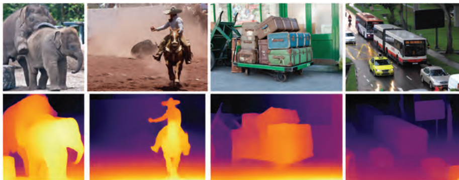
FIGURE 19.4: Predicting depth from single images is now a reliable technology. Top row shows images; bottom row , predicted depth representations. The predictor reports a_d\delta + b_d where \delta is disparity and a_d, b_d are per image constants. Orange is closer to the eye, purple is further from the eye. Notice: depth maps contain quite fine detail (eg the larger elephant’s trunk; where the rider contacts the horse; the grooves between suitcases); small depth gradients are well represented (eg along the cowboy’s arm); windows can cause confusion (eg window next to suitcases). Image credit: Figure 1 of “Towards Robust Monocular Depth Estimation: Mixing Datasets for Zero-shot Cross-dataset Transfer”, René Ranftl*, Katrin Lasinger*, David Hafner, Konrad Schindler, and Vladlen Koltun.
