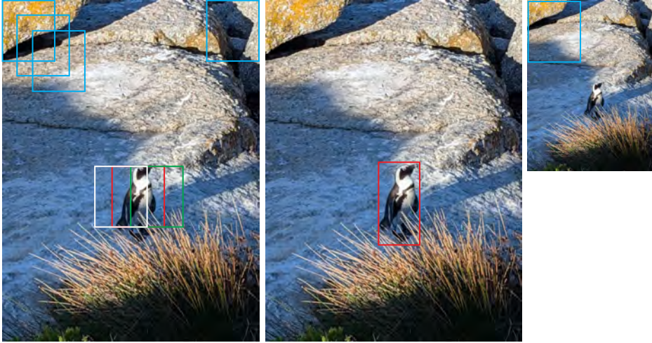
FIGURE 24.1: A simple penguin detector sweeps boxes across an image, passing each box to a classifier which computes a penguin score. On the right , quite rough localization (the red box is not exactly on the penguin) requires scoring a very large number of boxes (the blue boxes give some sense of the number). More accurate localization might require more boxes, but too many boxes create problems with efficiency and with the classifier. Because the classifier must be able to deal with boxes that don't closely hug the penguin, it must respond to the green and white boxes, too. You do not want to count three penguins, so use non-maximum suppression to produce the red box. You can then use bounding box regression to predict an update to the original box ( center ). If you want to find larger penguins, search a smaller version of the image ( right ). Image credit: Robert Forsyth's photograph of a Cape Penguin at Boulders Beach.
